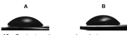
Figure 13 - Contact angle comparison between a membrane cleaned with pure water (A) and a fouled membrane (B), both from the flat-sheet batch.
