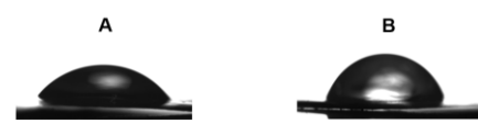
Figure 12 - Contact angle comparison between a membrane cleaned with pure water (A) and a membrane cleaned with Ultrasil 10 (B), both from the flat-sheet batch.
