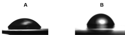
Figure 10 - Contact angle comparison between a fouled membrane (A) and a conditioned membrane (B), both from the flat-sheet batch.
