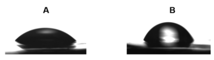
Figure 11 - Contact angle comparison between a fouled membrane (A) and a conditioned membrane (B), both from the spiral-wound module.
